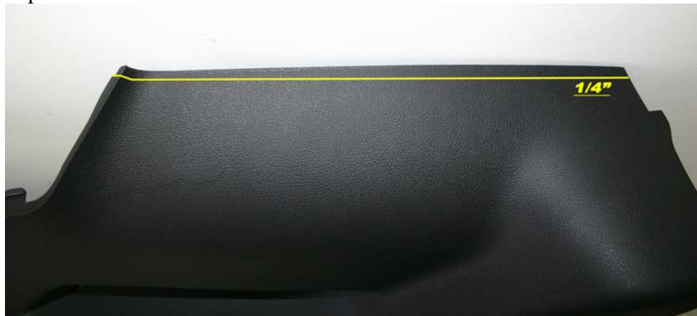
Lower panel shown above – approx. 1/4” coinciding with step in forward corner will need to be removed. If desired, cut can be tapered to zero removal going towards rear of vehicle.
